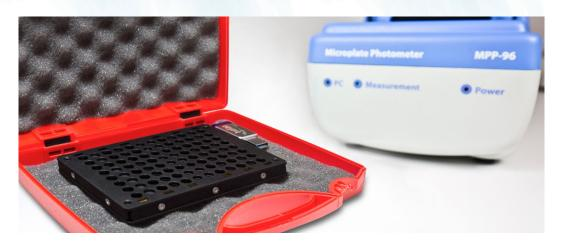
**OD Plate** is the measurement verification instrument for microplate photometer MPP-96 HiPo. The instrument is designed to verify the accuracy and precision of measurements of the photometer at six levels of nominal optical density: 0.3; 0.6; 1.0; 2.0; 3.0; 4.0 OD. The instrument is supplied with the following verification wavelength range: 405-700 nm.
