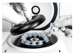
High-speed Mini-centrifuge Microspin 12 is a compact desktop centrifuge designed for biomedical laboratories.
